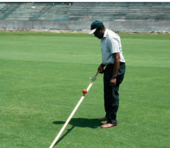
Dr Francis Lopez of the Sports Agronomy Research Unit using a modified stimp meter to assess turf speed at the Sir Vivian Richards Cricket Grounds in Antigua
