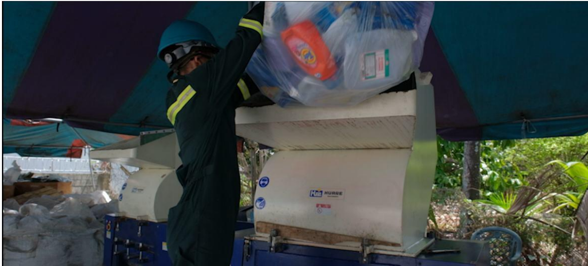
Plastic waste is shredded before being turned into lumber at a factory in Arima, Trinidad. UN News/ Brianna Rowe
